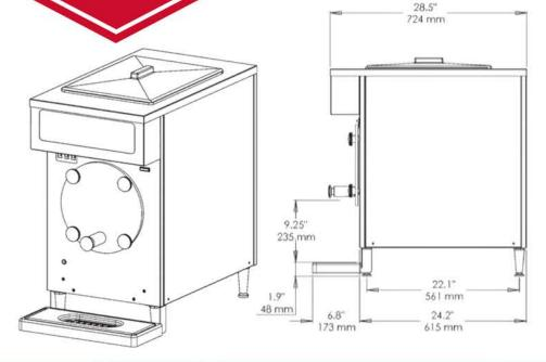
Minimum Wall Clearance Both Sides and Back 6 inches (152 mm)
